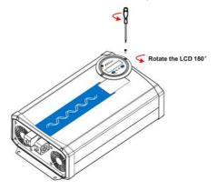
(2) Secure the screws of the LCD unit to the inverter.
